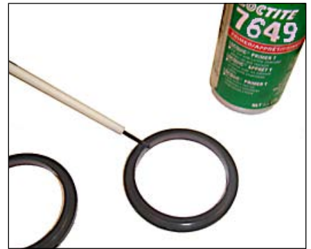
Figure 40. Applying Loctite primer to the outer step of the bearing cups
